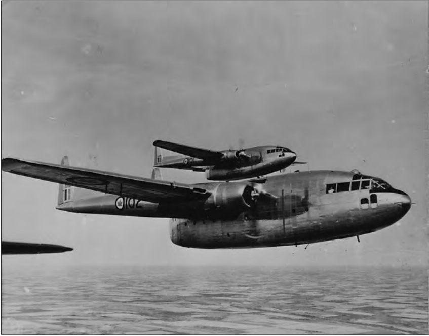
Early models of our C-119 lacked the lower dorsal tail fin (and the lateral stability) of the later models.
